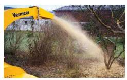
NO-COMPROMISE CHIPPING. Coupling the Kubota 48,1 hp (35,9 kW) engine to a 76 cm diameter 4-knife disc, the BC190xL can handle diametres up to 20 cm and discharges chips at an average distance from 10 to 12 metres - all this at 120 dB(A)!
