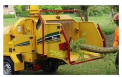
MARKET-LEADING INFEED. A large infeed opening of 203x305 mm in combination with a wide tapered infeed table provides the capacity to do the hard work for you.
